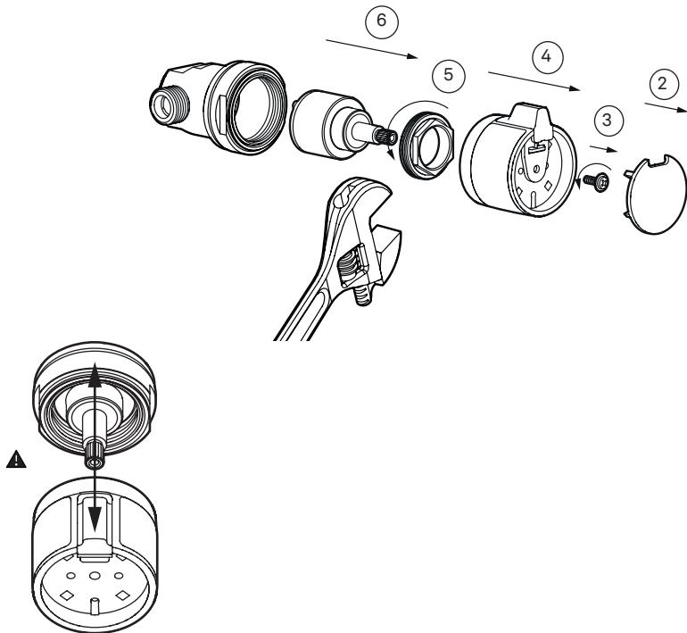
RENGÖRING AV INLOPPSSILAR/CLEANING THE INLET STRAINERS/RENGJØRING AV
