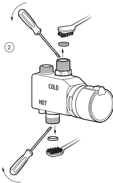
RENGÖRING AV TERmostatinSATS/CLEANING THE THERMOSTATIC CARTRIDGE/
