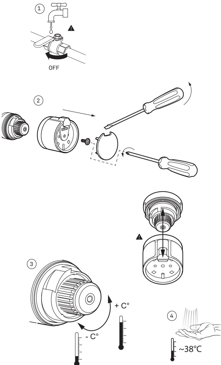
BYTE AV TERmostatInnSats/THERMOSTAT CARTRIDGE REPLACEMENT/BYTTE AV
